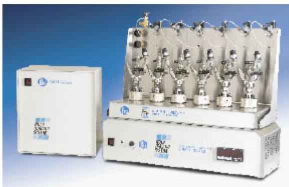
The 5000 MRS comes standard with six reactors, a gas distribution panel, magnetic stirring motor and stirring bars, and a 4871 Controller to monitor and control the parameters. For more information on the 5000 MRS [click here](#).
