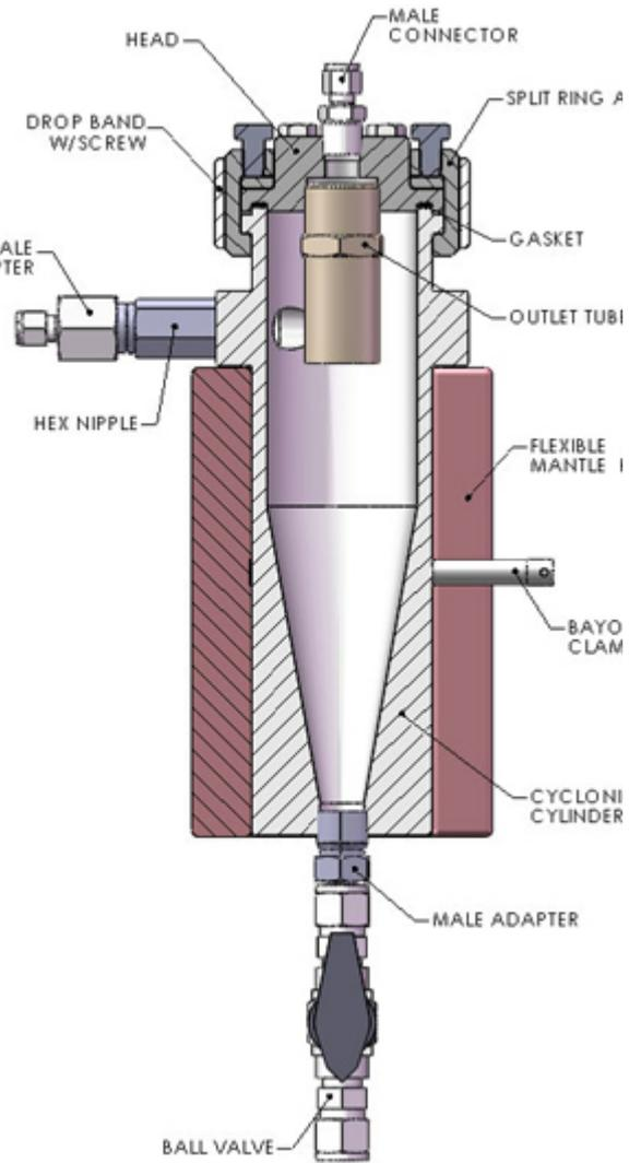
**Cutaway of the Cyclone Separator**
