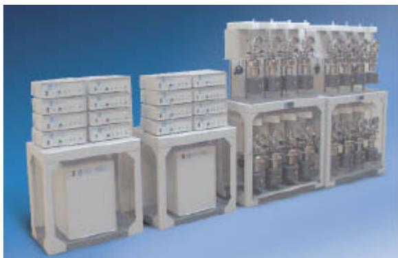
This system is a combination of sixteen standard 4560 Mini Reactors with heaters, valves, pressure gage and rupture disc assemblies and two 4871 Process Controllers with sixteen 4875 Power Controllers. It allows the user to run multiple reactions simultaneously, applying the principles of high-throughput experimentation. Individual variables that can be controlled are gas mixtures, liquids, catalysts or other solids, stirring speed, temperature, pressure and time.
