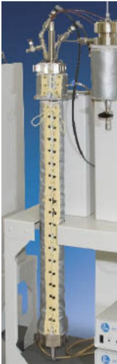
(Above) The Flexible Mantle Heater attaches in two pieces and provides even heating to the entire length of the reactor.
