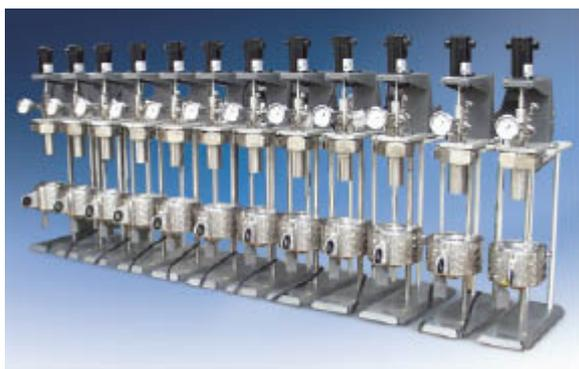
This system makes use of the lower cost 5500 High Pressure Compact Lab Reactors that feature a modified stand, aluminum block heaters, removable vessels and a standard gage block assembly. A control system (not pictured) automates the process, monitors the parameters and collects the data. Parr also provides a standard Multi Reactor System in the 5000MRS pictured below.
