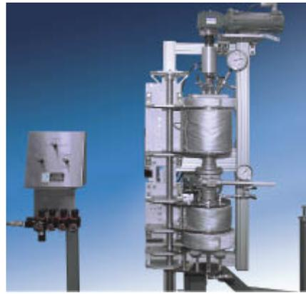
The reactor shown in the two images above and right has a five gallon capacity, and is used for stirring horizontally. Pneumatic controls on the left can tilt the system upright to open the bottom drain valve. The product is filtered and collected in a heated sample collection vessel below. This system is used for making fabric from biomass. Most synthetic fabric is made from oil.
