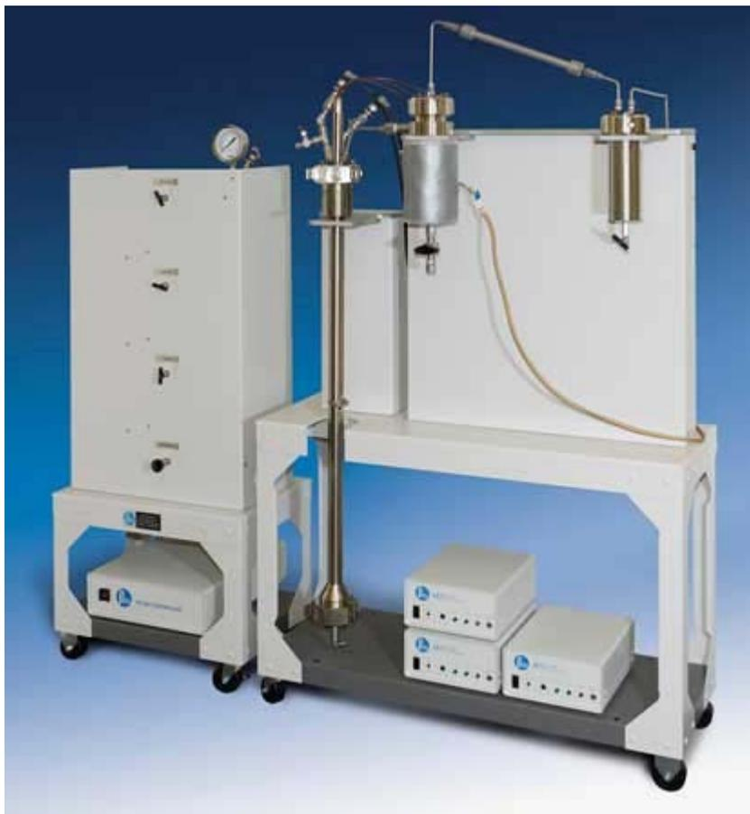
The Parr Fluidized Bed Reactor features the Reactor, a Heated Cyclone Separator, a Cooling Condenser, and a 600 mL Product Receiver.
